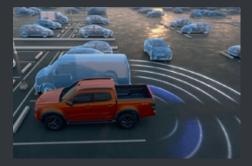
REVERSING CAMERA WITH REAR CROSS TRAFFIC ALERT (RCTA): Monitors your surrounding area while reversing into traffic, providing visual and audible warnings should an object approach from the left or right. (RCTA will disable when the genuine tow harness is connected).
