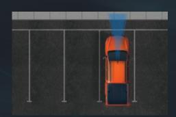
MISACCELERATION MITIGATION: In slow moving areas such as car parks, the stereo cameras determine whether the accelerator has been applied accidentally. Should a potential collision be detected, the accelerator is suppressed. (Automatic Transmission only).
