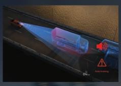
AUTONOMOUS EMERGENCY BRAKING (AEB): If your D-MAX detects a potential collision, emergency braking is applied automatically.
