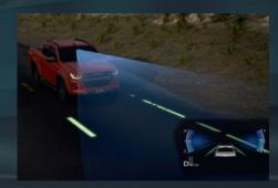
LANE KEEPING: Lane Keep Assist (LKA), Emergency Lane Keeping (ELK) and Lane Departure Prevention (LDP) work to help prevent collisions with other drivers should your D-MAX begin to drift across its lane. These features can also be disabled via the Lane Support System (LSS) switch.
