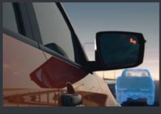
BLIND SPOT MONITOR (BSM): Provides a visual warning in your side mirrors when an obstacle is approaching in your blind spot. (BSM will disable when the genuine tow harness is connected).
