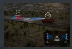
ADAPTIVE CRUISE CONTROL: Automatically adjusts your speed based on vehicles around you, including Stop and Go functionality when cruise control is activated. (Automatic Transmission only).
